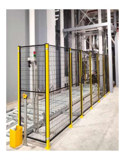
Vertical conveyors are used for conveying pallets to multi-level platforms and mezzanines. The pallets can thus be handled on several levels.
